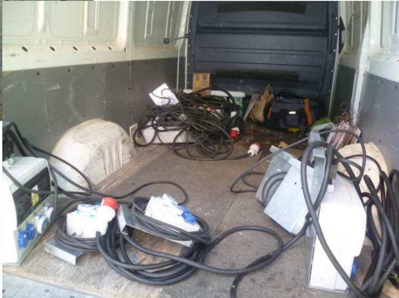
Service vehicle by e-rally organizer with cables, plugs and panels for charging column plant sufficient for 30 BEV
