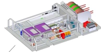
Water-cooled Traction converter
